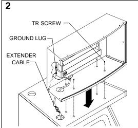
Connect Extender Cable to main harness and run it through holes in top of cabinet and bottom of Header Housing. Connect it to Lamp Assembly. Place ground lug over bottom left stud on Lamp Assembly and fasten with ESN nut. Align Housing with holes atop cabinet and fasten with tamper resistant screws.
